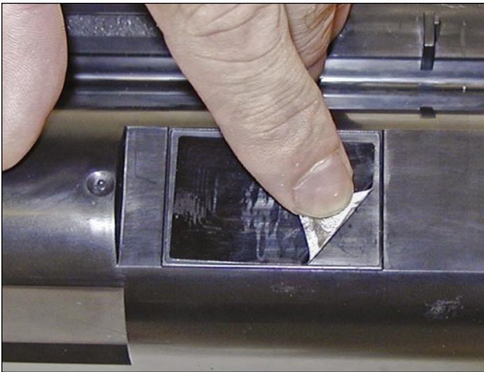
5. Replace the RF type chip (the chip is manufactured into the label).
