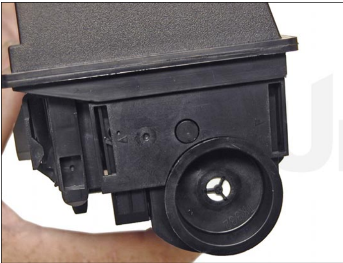
3. Re-install the fill plug.
